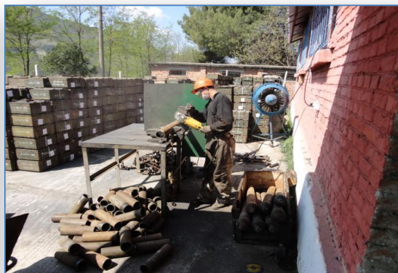
Mortar barrel cut in pieces
