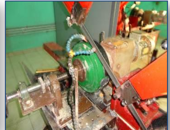
Remote cutting of metallic mine casing
