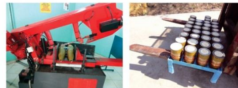
High-speed presses being processed using an industrial band saw (left), and the resulting opened shells being transported for the removal of explosive (right). © NMSA
