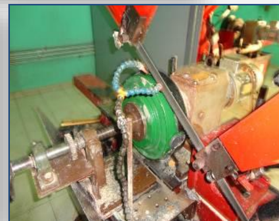
Remote cutting of metallic mine casing
